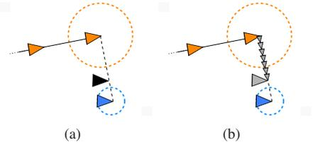
Fig. 4. External (a) and internal (b) fusion mechanisms for trajectory bending. The uncertainty in the last absolute pose is depicted by the orange circle and the uncertainty in the desired pose by the blue circle. The optimal combination of the last absolute pose and the desired pose is shown by the black triangle in (a). In (b) the local updates end at the large gray triangle which has the same position as the optimal combination of the last absolute pose and the desired pose.
